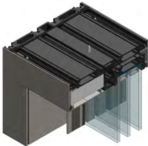
Detail S52 Deckenschiene
